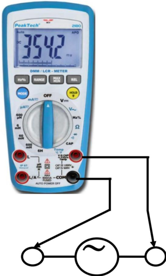
**Warning!** When you connect the test probes to an AC outlet/ mains voltage , do not turn the rotary selector switch to another range. It could damage the meter's internal components or injure you.
