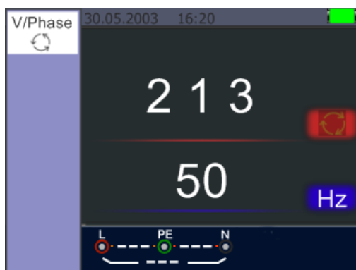
Phase Sequence – When connected in counter-clockwise manner
