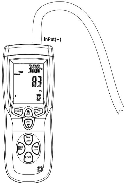
3. With the tubing open to ambient conditions press the “HOLD-button” and hold for 2 seconds to zero out the display.
