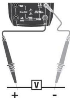
1. Set the function switch to the  $mV \sim$ -position.
