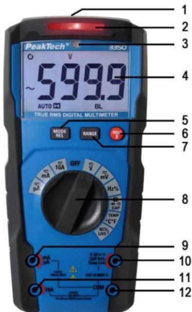
1. Non-contact voltage tester (sensor)
