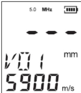
Adjusting the sound speed within the unit
