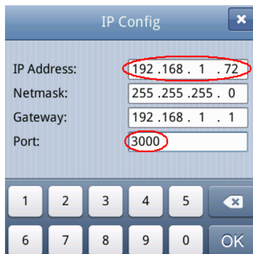
Figure 0-4 Set the network parameters of the oscilloscope
