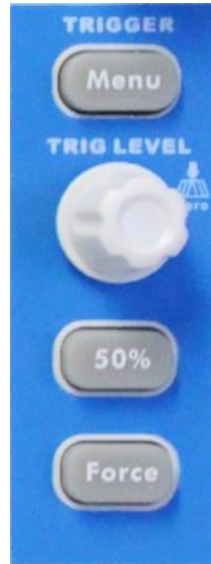
Figure 0-12 Trigger Control Zone
