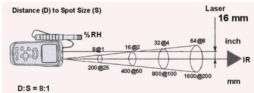
D = Distancefactor (avoid expose-laser radiation is emitted from this aperture) approx. 8 : 1
