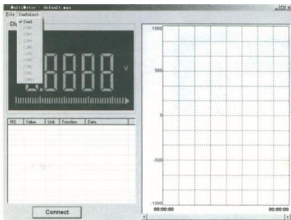
8. Power on the DMM and then push the USB button more than 3 seconds to inert to the Communication mode. The "PC-Link" symbol will be displayed on the LCD.
