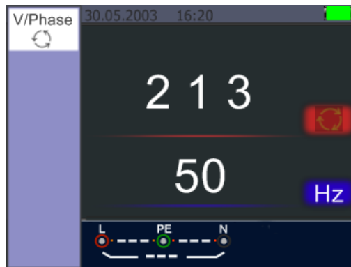
Phase Sequence – When connected in counter-clockwise manner
