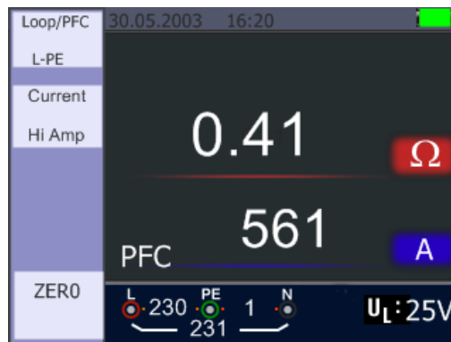
Hi Amp LOOP – Measurement finished
