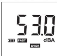
When the sound level will be detect over the set value, the unit will alarm & LED flash (01 = alarm mode) or only LED flash (02 = alarm mode). Alarm will stop continue 15 seconds. After stop 5 seconds. If unit detect the sound level over set value, the unit will alarm again. In this mode the unit will not automatic power off. Press “MAX/MIN”-key again cancel alarm mode. See Fig. 5.
