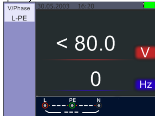
Standby screen for the Voltage and Frequency
