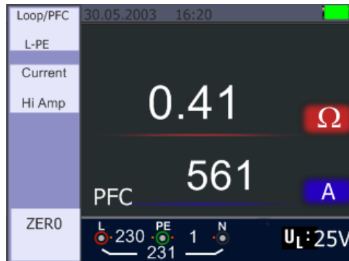
Hi Amp LOOP – Measurement finished
