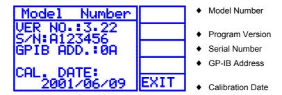
[**F5**] EXIT button: Pressing the [**F5**] button returns the to the counter display.
