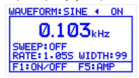
[Figure 6] LCD Display (SWEEP display mode)
