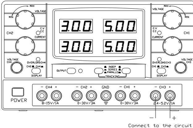
1. Connect the power supply to the power source.
