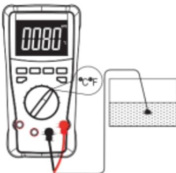
4. Read the temperature in the display. The digital reading will indicate the proper decimal point and value.
