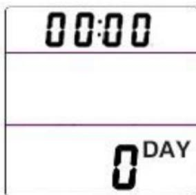
While the time is being recorded, a colon (:) flashes on the display. The first two numbers indicate the hours, while the last two numbers show the minutes.
