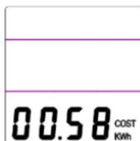
Press and hold the SET button to set the electricity price Cost/KWh. After entering the unit price setting, the first digit flashes, press the up and down buttons to adjust the value, briefly press the SET button to select the next digit. To finish the setting, wait 10 seconds until the display stops flashing or hold the SET button for 3 seconds, your entry is now saved.
