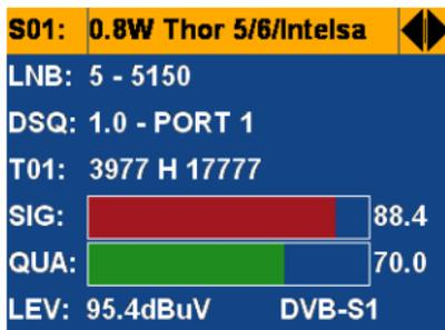
1. Click OK to display the list of transponder with the corresponding level and signal quality.
