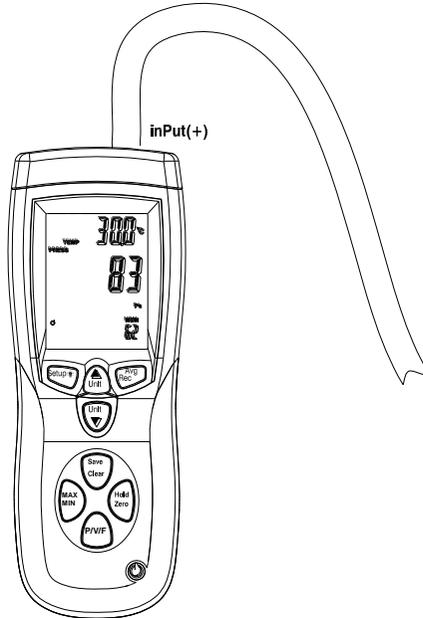
3. With the tubing open to ambient conditions press
