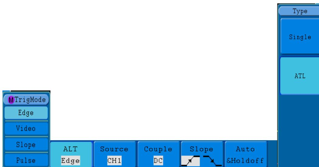
**FIG. 34 Alternate Trigger** (Trigger Type: Edge)
